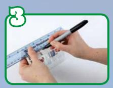
Stick a piece of tape from the top to the bottom of the rain catcher. Using a ruler, draw a line and mark 10 centimetres starting with 0 at the bottom moving up to 10 at the top.
